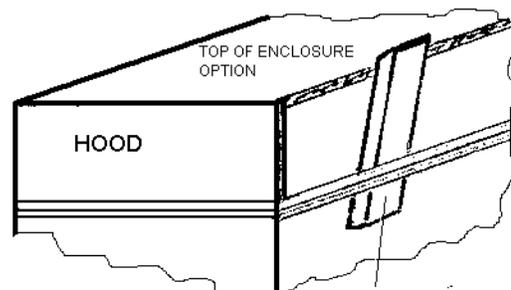
A RECTANGULAR FUNNEL CAN BE MADE OUT OF THIN PLASTIC AVAILABLE AT MOST HOBBY SHOPS. AN EXTENSION COULD ALSO BE ADDED TO CURRENT FUNNEL.
